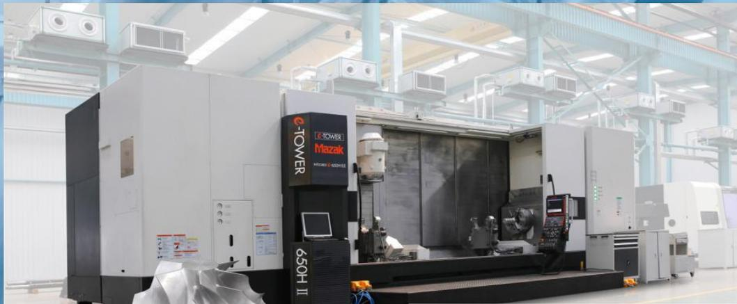
Mazak turning and milling compound machining
